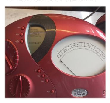
measures changes in skin resistance and displays this with a needle. The original circuit was just a Whetstone Bridge, and has since been "upgraded" by adding a digital display driven by a microprocessor, capable of counting the number of movements of the needle.
